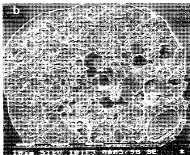
Fig. 2. Scanning electronic micrographs of the fractured PLGA-PVA composite microspheres showing the internal structure and distribution of the PVA nanoparticles inside the PLGA microspheres. (a) a group of the fractured composite microspheres and (b) an enlarged view of a fractured composite microsphere.
